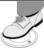
Walk over fittings max static weight 2000kg
