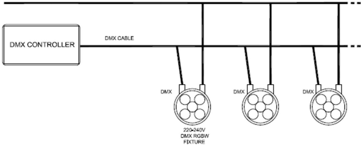
DMX/RDM is a robust and reliable system for lighting control. However, if not implemented correctly, problems can arise such as random flashing of lights, erratic operation and delays in responding to commands. This document explains the best practices in DMX wiring.
